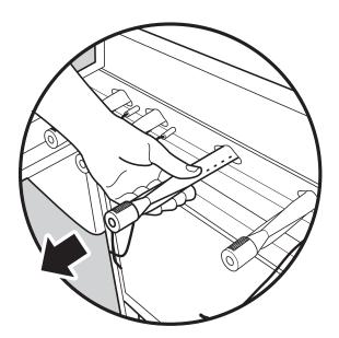
**△CAUTION:** The burner openings (1) must be positioned properly over the valve orifices (2).
